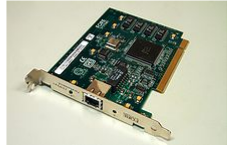
An ATM network interface in the form of an accessory card. A lot of network interfaces are built-in.
