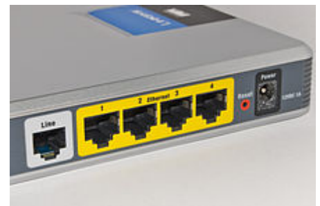
A typical home or small office router showing the ADSL telephone line and Ethernet network cable connections
