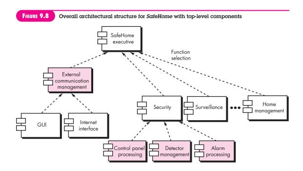
Internet interface. This information is managed by a *SafeHome* executive component that selects the appropriate product function (in this case security). The *control panel processing* component interacts with the homeowner to arm/disarm the security function. The *detector management* component polls sensors to detect an alarm condition, and the *alarm processing* component produces output when an alarm is detected.
