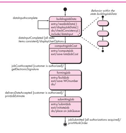
(mode of behavior) of the object. To understand the dynamic behavior of an object, you should examine all use cases that are relevant to the design class throughout its life. These use cases provide information that helps you to delineate the events that affect the object and the states in which the object resides as time passes and events occur. The transitions between states (driven by events) are represented using a UML statechart [Ben02] as illustrated in Figure 10.9.
