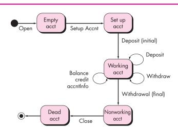
Still more test cases could be derived to ensure that all behaviors for the class have been adequately exercised. In situations in which the class behavior results in a collaboration with one or more classes, multiple state diagrams are used to track the behavioral flow of the system.
