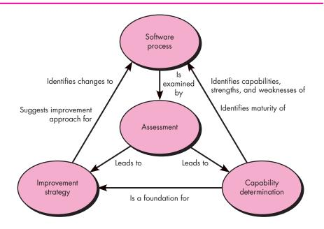
An SPI framework assesses the "maturity" of an organization's software process and provides a qualitative indication of a maturity level. In fact, the term "maturity model" (Section 30.1.2) is often applied. In essence, the SPI framework encompasses a maturity model that in turn incorporates a set of process quality indicators that provide an overall measure of the process quality that will lead to product quality.
