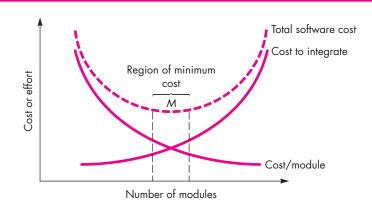
same set of requirements, more modules means smaller individual size. However, as the number of modules grows, the effort (cost) associated with integrating the modules also grows. These characteristics lead to a total cost or effort curve shown in the figure. There is a number, M, of modules that would result in minimum development cost, but we do not have the necessary sophistication to predict M with assurance.
