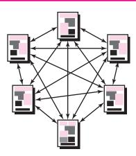
(in this case, Web pages) are designed so that they may pass control (via hypertext links) to virtually every other component in the system. This approach allows considerable navigation flexibility, but at the same time, can be confusing to a user.
