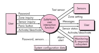
The function manages user interaction, accepting a user password to activate or deactivate the system, and allows inquiries on the status of security zones and various security sensors. The function displays a series of prompting messages and sends appropriate control signals to various components of the security system.
