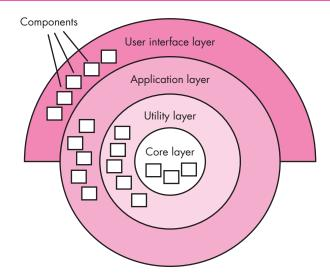
**Layered architectures.** The basic structure of a layered architecture is illustrated in Figure 9.4. A number of different layers are defined, each accomplishing operations that progressively become closer to the machine instruction set. At the outer layer, components service user interface operations. At the inner layer, components perform operating system interfacing. Intermediate layers provide utility services and application software functions.
