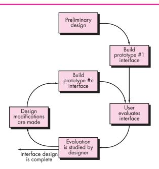
The prototyping approach is effective, but is it possible to evaluate the quality of a user interface before a prototype is built? If you identify and correct potential problems early, the number of loops through the evaluation cycle will be reduced and development time will shorten. If a design model of the interface has been created, a number of evaluation criteria [Mor81] can be applied during early design reviews:
