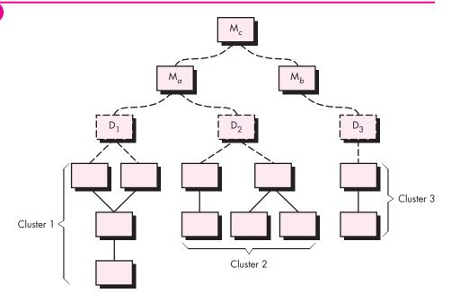
As integration moves upward, the need for separate test drivers lessens. In fact, if the top two levels of program structure are integrated top down, the number of drivers can be reduced substantially and integration of clusters is greatly simplified.
