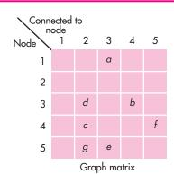
Referring to the figure, each node on the flow graph is identified by numbers, while each edge is identified by letters. A letter entry is made in the matrix to correspond to a connection between two nodes. For example, node 3 is connected to node 4 by edge b.
