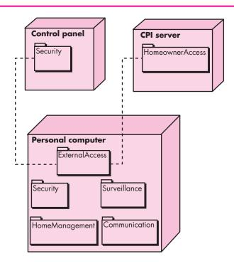
the software. For example, the elements of the *SafeHome* product are configured to operate within three primary computing environments—a home-based PC, the *SafeHome* control panel, and a server housed at CPI Corp. (providing Internet-based access to the system).
