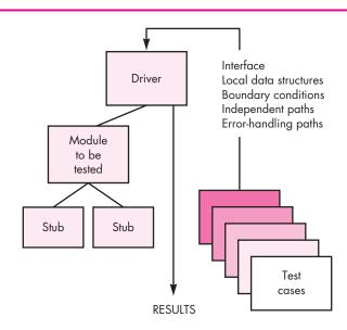
relevant results. *Stubs* serve to replace modules that are subordinate (invoked by) the component to be tested. A stub or "dummy subprogram" uses the subordinate module's interface, may do minimal data manipulation, prints verification of entry, and returns control to the module undergoing testing.
