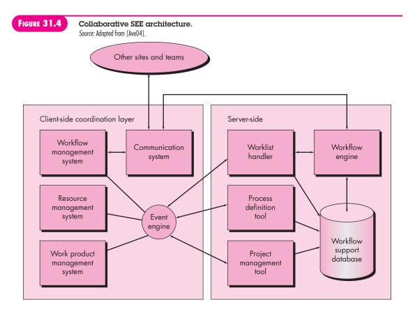
On the server side, four components share a workflow support database. The components implement the following functions:
