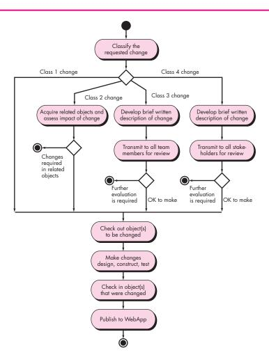
change can be made without requiring significant changes to other objects, modification occurs without additional review or documentation. If substantive changes are required, further evaluation and planning are necessary.
