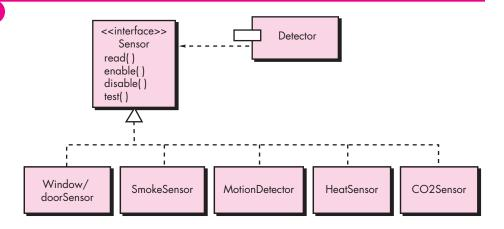
contradiction, but it represents one of the most important characteristics of a good component-level design. Stated simply, you should specify the component in a way that allows it to be extended (within the functional domain that it addresses) without the need to make internal (code or logic-level) modifications to the component itself. To accomplish this, you create abstractions that serve as a buffer between the functionality that is likely to be extended and the design class itself.
