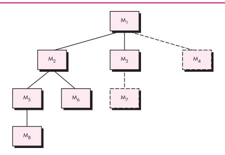
(main program). Modules subordinate (and ultimately subordinate) to the main control module are incorporated into the structure in either a depth-first or breadth-first manner.
