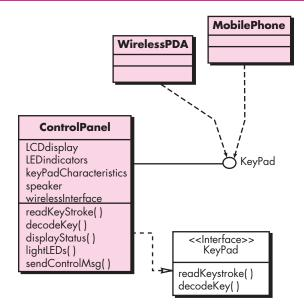
is characterized as a *realization*. That is, part of the behavior of **ControlPanel** will be implemented by realizing **KeyPad** operations. These operations will be provided to other classes that access the interface.
