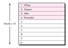
shown in Figure 21.7. It represents the table used by an operating system to hold the names of the users of the system. Other examples of tables include the collection of names of staff in a payroll system, the collection of names of computers in a network communications system, and the collection of destinations in a system for producing transportation timetables.
