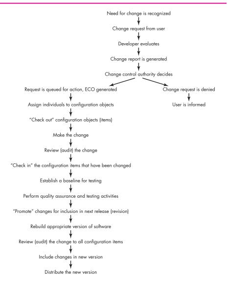
the object(s) to be changed can be "checked out" of the project database (repository), the change is made, and appropriate SQA activities are applied. The object(s) is (are) then "checked in" to the database and appropriate version control mechanisms (Section 22.3.2) are used to create the next version of the software.
