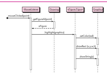
the *getFigureAt()* method call's return is shown labeled with the name of the object that was returned. A common practice, as we have done in Figure A1.7, is to leave off the return arrow when a void method has been called, since it clutters up the diagram while providing little information of importance. A black circle with an arrow coming from it indicates a *found message* whose source is unknown or irrelevant.
