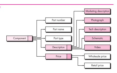
values) are represented as unshaded rectangles. Content objects are represented as shaded rectangles. In the figure, **description** is defined by five content objects (the shaded rectangles). In some cases, one or more of these objects would be further refined as the data tree expands.
