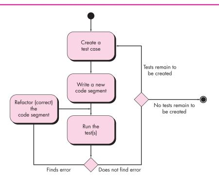
In TDD, tests drive the detailed component design and the resultant source code. The results of these tests cause immediate modifications to the component design (via the code), and more important, the resultant component (when completed) has been verified in stand-alone fashion. If you have further interest in TDD, see [Bec04b] or [Ast04].
