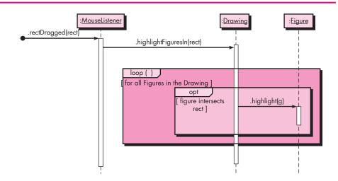
**Figure** intersects the rectangle, the **Figure** is asked to highlight itself. The phrases in square brackets are called *guards*, which are Boolean conditions that must be true if the action inside the interaction frame is to continue.
