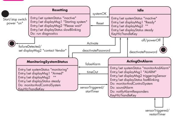
activated (i.e., alarm system is turned on), a transition to the **Monitoring-SystemStatus** state occurs, display messages are changed as shown, and the process *monitorAndControlSystem* is invoked. Two transitions occur out of the **MonitoringSystemStatus** state—(1) when the system is deactivated, a transition occurs back to the **Idle** state; (2) when a sensor is triggered into the **ActingOnAlarm** state. All transitions and the content of all states are considered during the review.
