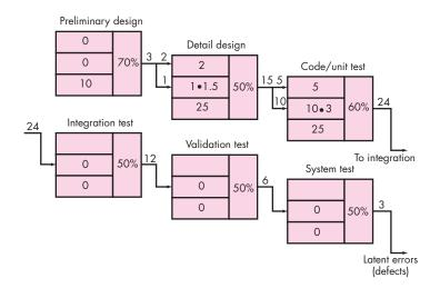
error (1.5 cost units for design, 6.5 cost units before test, 15 cost units during test, and 67 cost units after release). Using these data, the total cost for development and maintenance when reviews are conducted is 783 cost units. When no reviews are conducted, total cost is 2177 units—nearly three times more costly.
