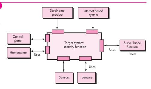
function in Figure 9.6. The surveillance function is a *peer system* and uses (is used by) the home security function in later versions of the product. The homeowner and control panels are actors that are both producers and consumers of information used/produced by the security software. Finally, sensors are used by the security software and are shown as subordinate to it.
