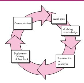
formats). The quick design leads to the construction of a prototype. The prototype is deployed and evaluated by stakeholders, who provide feedback that is used to further refine requirements. Iteration occurs as the prototype is tuned to satisfy the needs of various stakeholders, while at the same time enabling you to better understand what needs to be done.
