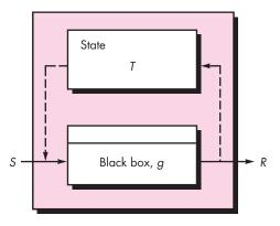
Many of the concepts introduced for object-oriented systems are also applicable for the black box. Data abstractions and the operations that manipulate those abstractions are encapsulated by the black box. Like a class hierarchy, the black-box specification can exhibit usage hierarchies in which low-level boxes inherit the properties of those boxes higher in the tree structure.
