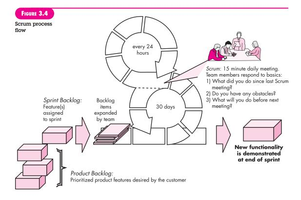
framework activity, work tasks occur within a process pattern (discussed in the following paragraph) called a *sprint*. The work conducted within a sprint (the number of sprints required for each framework activity will vary depending on product complexity and size) is adapted to the problem at hand and is defined and often modified in real time by the Scrum team. The overall flow of the Scrum process is illustrated in Figure 3.4.
