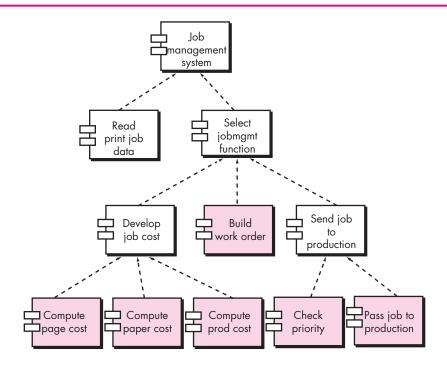
would be derived during requirements modeling. Assume that these are mapped into an architecture shown in Figure 10.2. Each box represents a software component. Note that the shaded boxes are equivalent in function to the operations defined for the **PrintJob** class discussed in Section 10.1.1. In this case, however, each operation is represented as a separate module that is invoked as shown in the figure. Other modules are used to control processing and are therefore control components.
