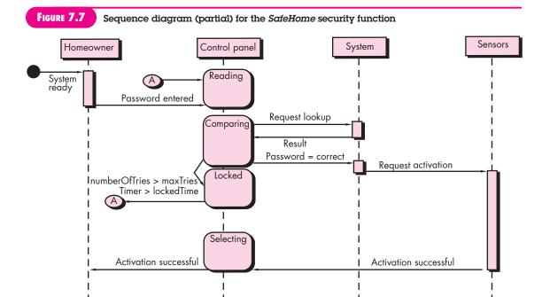
creates a sequence diagram—a representation of how events cause flow from one object to another as a function of time. In essence, the sequence diagram is a short-hand version of the use case. It represents key classes and the events that cause behavior to flow from class to class.
