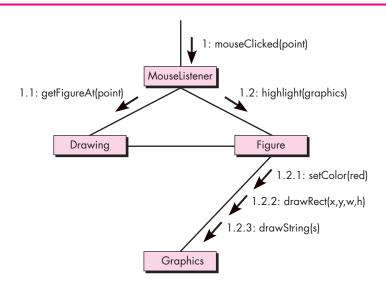
A communication diagram, illustrated in Figure A1.10, displays the same actions shown in the sequence diagram in Figure A1.7.
