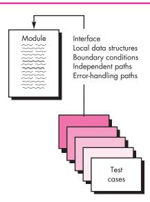
guide, important control paths are tested to uncover errors within the boundary of the module. The relative complexity of tests and the errors those tests uncover is limited by the constrained scope established for unit testing. The unit test focuses on the internal processing logic and data structures within the boundaries of a component. This type of testing can be conducted in parallel for multiple components.
