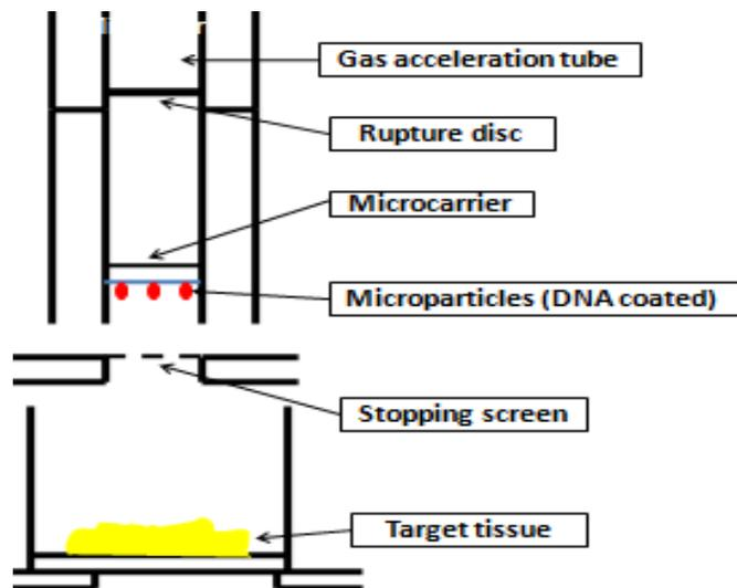
Figure 5-3.1.3(b). Working system of particle bombardment gun.
