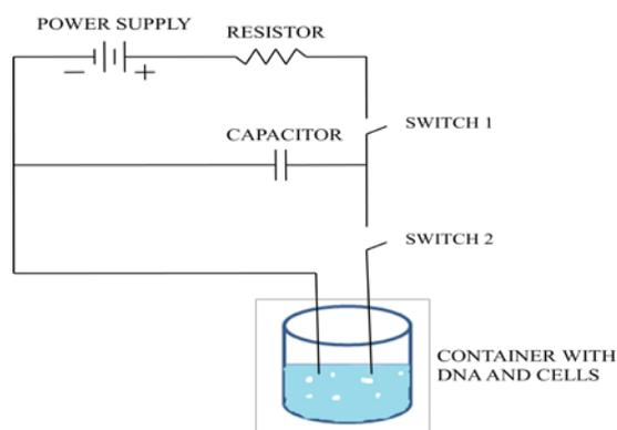
**Figure 5-3.1.1(a). The basic circuit setup of the electroporation apparatus.**
