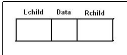
Fig. (11) A node structure of a binary tree
