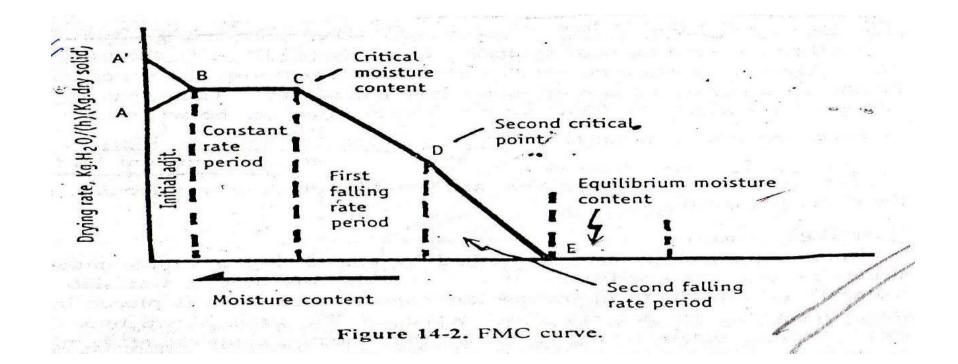
The time corresponding to AB represents the initial adjustment period. During this period, the solids absorb heat and the temperature increases. At the same time, the moisture begins to evaporate and thus tends to cool the drying solid. After some time, the temperature stabilises (heating and cooling rates become equal). This temperature is equal to the vet bulb temperature of the drying air and is referred by the point B.
